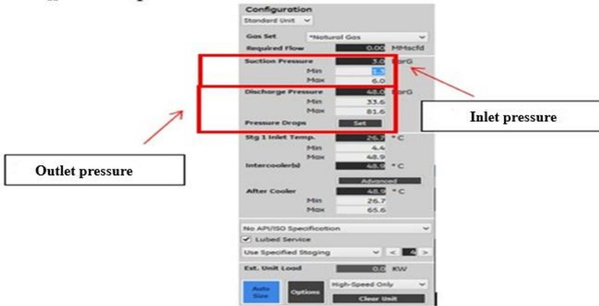
Figure 6: Input of Inlet and Outlet Gas Parameters
